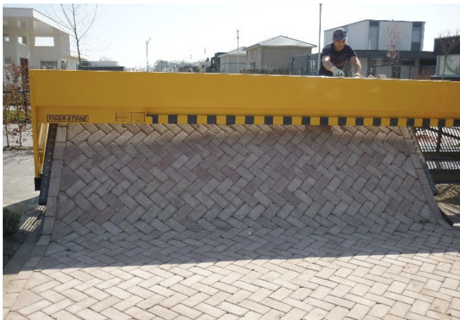
Figure 72 - Paver Laying Machine (Detroit News)
