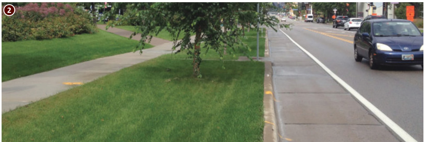
Figure 50 - Basic Roadside Swale (NACTO)
