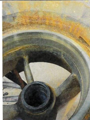
Suction stage, "grooving" evidence & minor ring wear
