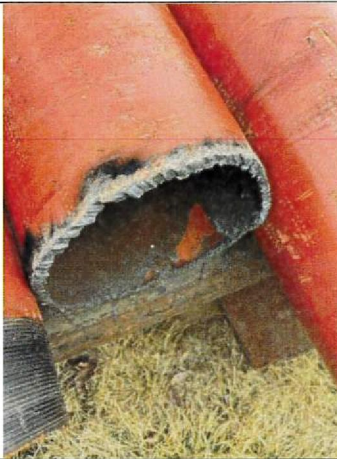
Cut pipe due to power tongs not being able to break loose.
