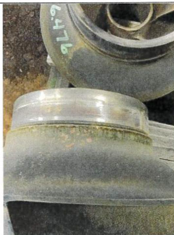
Impeller ring discoloration potentially caused by heat, w/ grooves & minor wear
