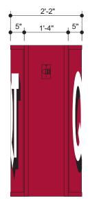
All Sign Modules constructed with removable alum. face retainers and clear acrylic, .177" thickness, face panels with 2nd surface painted background colors and graphics.
