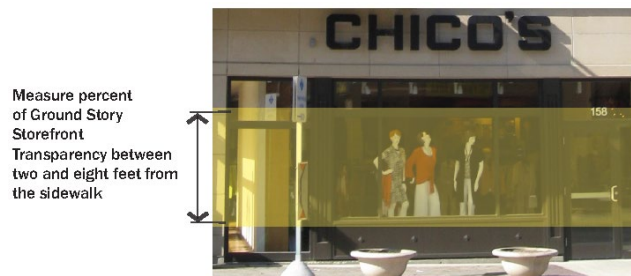
Figure 3.27 Measuring Ground Floor Transparency on a Storefront Base
