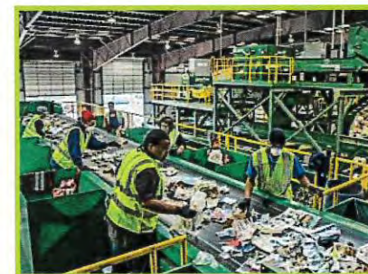
All trash generated at QT stores in Tulsa is sent to a materials recycling facility (MRF) where plastic, glass, metal, cardboard, and paper products are separated for recycling.
