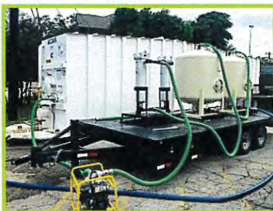
Carbon filter trailer used to treat contaminated groundwater before being discharged into the storm sewer system.
