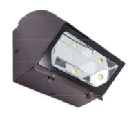
WallPack: The exterior wall packs will be replaced with a new LED fixture. This new fixture will eliminate the need for both the metal halide lamp and ballast. This upgrade will significantly reduce the consumed watts while not compromising illumination. Additionally, this fixture can be installed to wall wash or forward throw lights, mitigating neighbor complaints.
