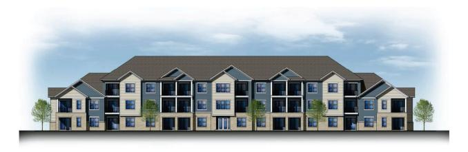
The petitioner has also provided architectural renderings (illustrated above) which shows the intended appearance of the main structure. The exterior will have a combination a masonry brick, masonry headers, composite siding and trim, vinyl windows and doors, aluminum railings, and asphalt shingles. While not required for the rezoning and variance process, staff wanted to ensure the petitioner was aware of the appearance code standards required by the City.
