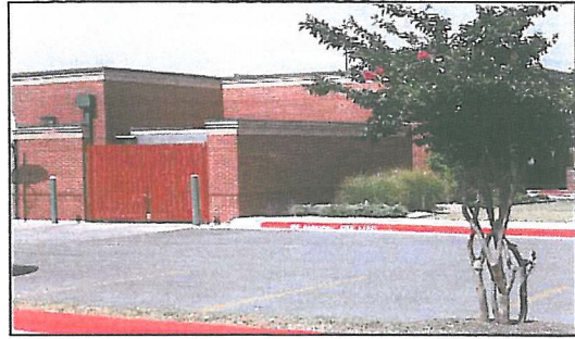
Screen dumpsters with walls and materials that match architecture of primary building
