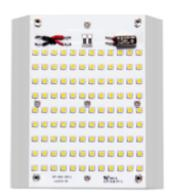
LED Panel Retrofit: HID lighting can be replaced with a high wattage LED panel retrofit. The ballast and metal halide will be removed, and an LED panel will be fitted inside the existing housing. This improvement will drastically reduce the consumed watts of the fixture. Heat dissipation is mitigated with an internal DC fan that keeps the LED cool and extends the life.
