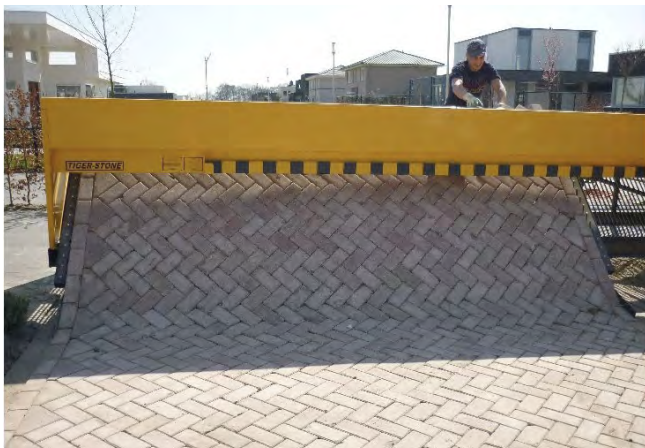
Figure 72 - Paver Laying Machine (Detroit News)
