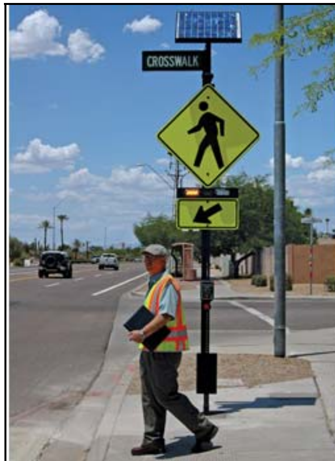
Photo 3. Sample RRFB Installation in Phoenix, AZ
