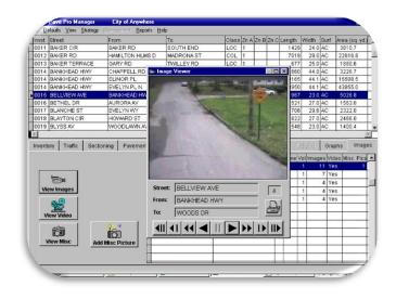
IMS uses an automated image capture process that is cost effective and provides for a user-defined frequency for the number of pictures per section.
